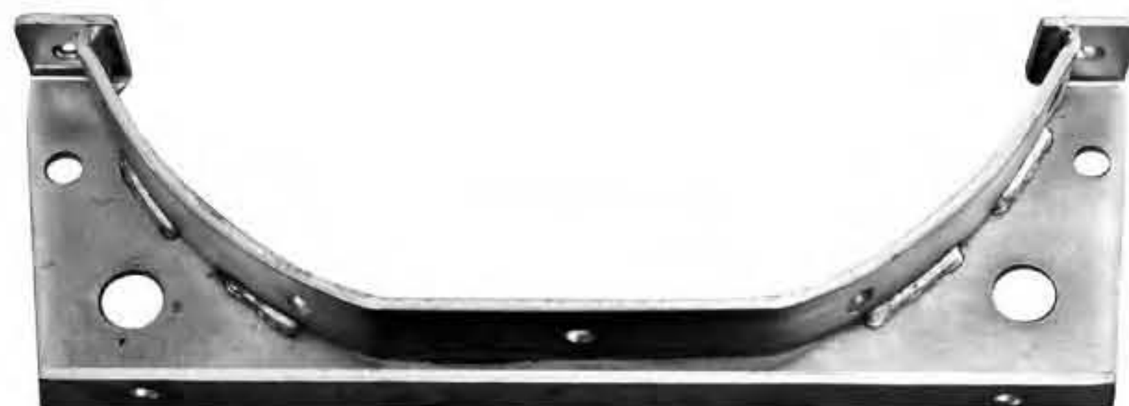
REAR TRANS SUPPORT TO BE USED WITH URETHANE OR STOCK CRADLE MOUNTS
