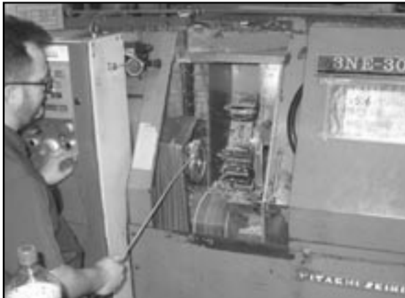
SCAT pulleys are machined from billet aluminum and micropolished to a fine luster.
