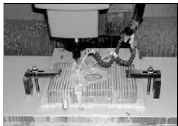
SCAT aluminum oil sump are CNC machined to exact tolerances for a perfect fit and seal.
